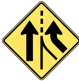
Added Lane (from right, no merging required)
